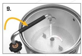
Place the tempered glass lid (27) on the boiler. Screw the recirculation pipe (25) onto the discharge pipe (17). Make sure it is threaded on correctly. The silicone hose (26) should go through the hole in the glass lid and rest on the top perforated plate (38). NOTE: The clips should not be used to secure the lid, these are for when using the distilling attachment only.
