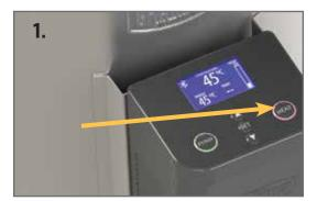
Once the inner basket (34) has been locked in place to drain, you can set the G30 to boil to allow the wort to come up to temperature while sparging, which saves time. NOTE: Do not let it come to a boil while the inner basket is still on top otherwise you could cause a boil over.
