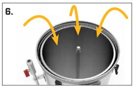
Once the control box indicates the correct mash temperature (from your recipe), slowly add the grain to the inner basket (34), stirring well to avoid any dry clumps.
