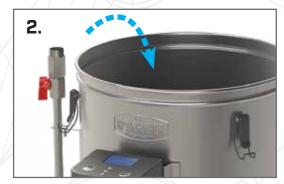
Add the required amount of mash water to the boiler body (28). Make sure the inner basket (34) is removed so that the scale on the inside of the boiler is visible.
