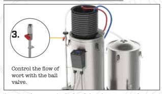
Ensure no hoses are kinked and that the water can flow freely, then gradually turn on your cooling water and adjust the flow rate. Allow the cooling water to flow for two minutes then turn on the pump. Once the cold wort out hose runs cool, switch the pump off and place the end of the hose inside your cleaned and sanitised fermenter and switch the pump back on. Always try to keep the fermenter opening covered to avoid contamination while transferring your wort.
