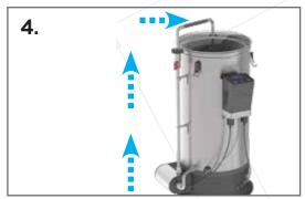
Empty the cleaner and fill the boiler with clean cold water. Scrub the bottom and sides of the boiler with a soft bristle brush. Make sure to recirculate water through the counterflow chiller and recirculation pipe.
