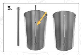
Place the grain stopper (35) into the top overflow pipe (39). the grain stopper has a rolled edge to show the maximum level the top overflow pipe can extend without pulling it off.
