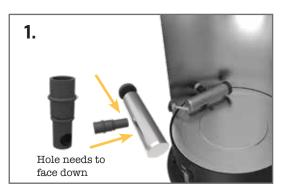
To install the filter (14) insert the silicone tube into the hole of the filter, with the hole in the tube facing down. Push it in so that the filter sits in the groove in the silicone tube. Push the round silicone piece onto the open side of the filter. Now install the filter onto the boiler by pushing the silicone tube over the filter inlet (13).
