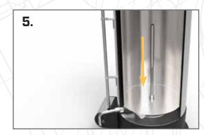
Push the top overflow pipe (39) over the bottom overflow pipe (40). Make sure the wire springs are facing down.
