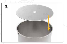
Push the bottom perforated plate (42) all the way down into the inner basket (34). Push down on the sides to ensure it is level. NOTE: You need to be firm when pushing it down, it is designed to be tight fitting. Wet the inside of the grain basket or run some grain dust around it so the silicone seal doesn't stick and it is easier to insert
