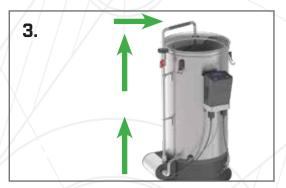
After 5 minutes remove the counterflow chiller and connect the recirculation pipe (25). Recirculate the cleaner for another 10 minutes.
