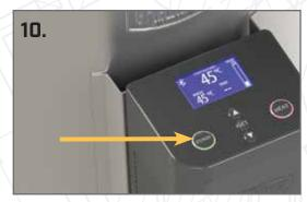
Switch on the pump. The wort flowing through the recirculation pipe should fill up on top of the top perforated plate.
