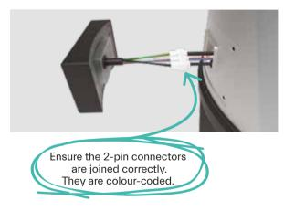
**NOTE:** Ensure correct orientation of the connectors as per the diagram below.
