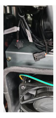
Located the Level sensor cable and disconnect the connector.
