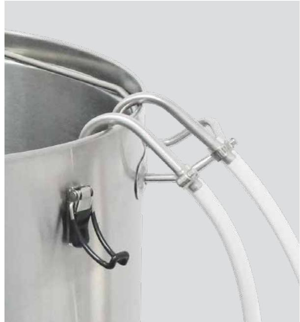
3. Check which hose is connected to the immersion chiller where the coil goes straight to the bottom (see image below). On the other end of that hose, attach the tap adapter and push the final clamp onto the end.
