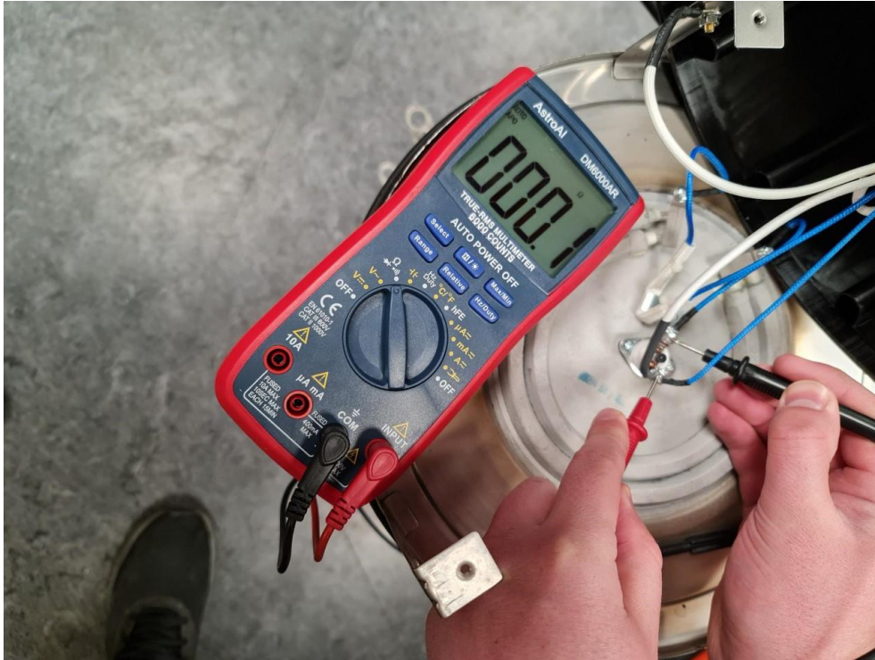
Figure 1, testing the continuity of the reset switch.
